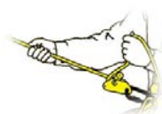
Figure 9-2. Proper use of Y-lanyard
