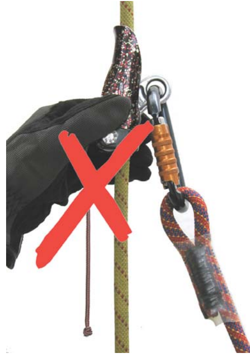
Figure 9-8. Do not handle body of back-up device.
