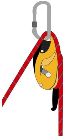
Figure 10-3. Redirecting the rope for extra friction for lowering operations
