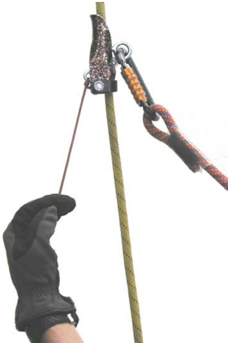
Figure 9-6. Moving back-up device down using tow string.
