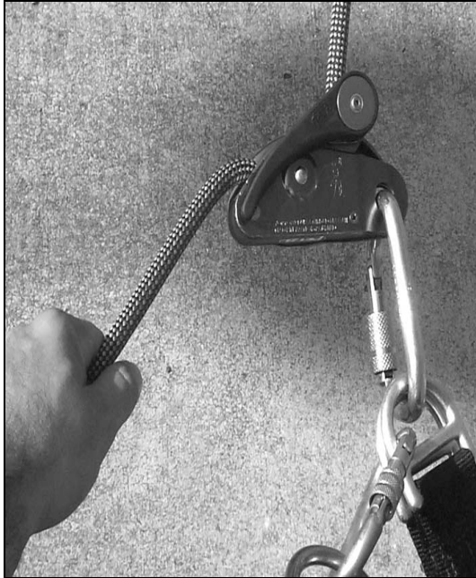
Figure 9-3: Belay device connected to anchor.
